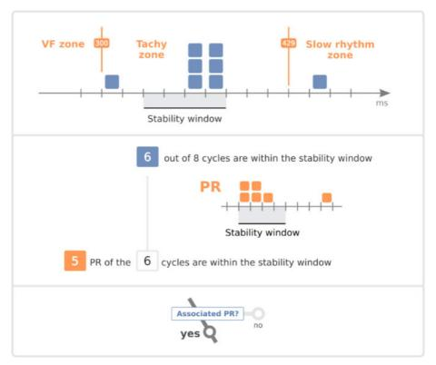
The PR intervals of the 6 stable RR intervals are analysed: the highest number of PR intervals fitting within the stability window is 5: the majority is reached ( $5/6 \ge 75\%$ ), the PR association is confirmed.
