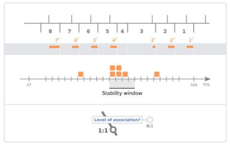
Figure 12: The max number of PR intervals within a stability window is 5, which represents at least 75% of the total PR intervals (7): the association level is 1:1.
