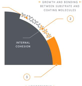
→ HOMOGENEOUS ← COATING PROVIDING MAXIMUM SLIDE
